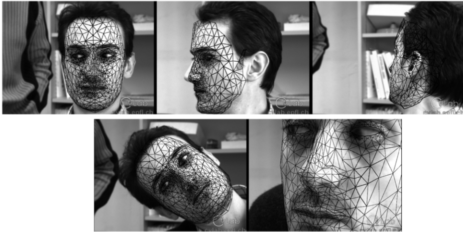
Figure 3: Face tracking using interest points and one reference image shown on the top left.
