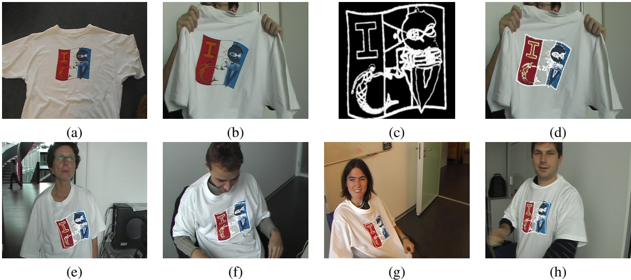
Figure 6: Real-time detection of a deformable object. Given a model image (a), the algorithm computes a function mapping the model to an input image (b). To illustrate this mapping, the contours of the model (c) are extracted using a simple gradient operator and used as a validation texture which is overlaid on the input image using the recovered transformation (d). Additional results are obtained in different conditions (e to h). Note that in all cases, the white outlines project almost exactly at the right place, thus indicating a correct registration and shape estimation. The registration process, including image acquisition, takes about 80 ms and does not require any initialization or a priori pose information.
